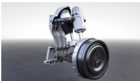
AUMOVIO Corner Module: Compact by-wire chassis unit that fits in a passenger car
